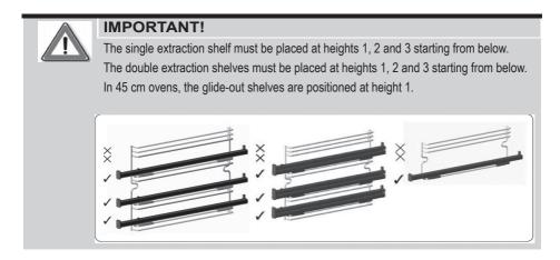
□ Hook the clip on the top rail at the desired level.
